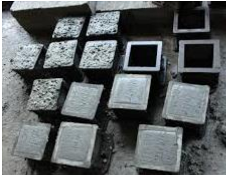
Figure 4. cast mortar cubes
