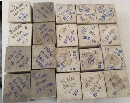
Figure 5. Ambient & Oven cured mortar cubes
