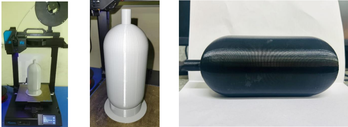
Figure 1. 3D printing of ABS & PET-G hydrogen storage cylinder.
