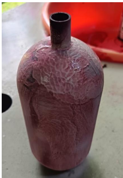
Figure 29. Dye penetrant test of ABS material
