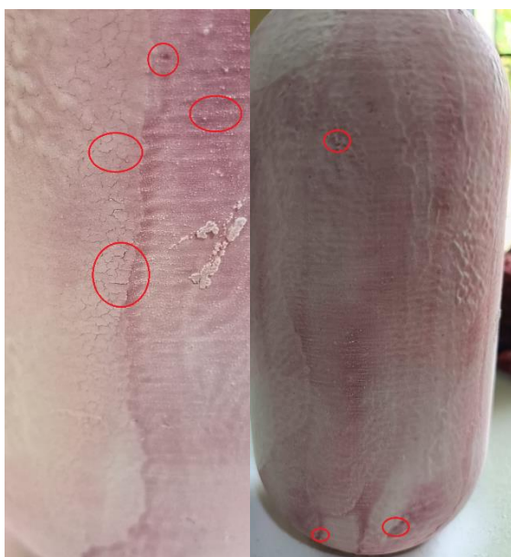
Figure 28. Defect finding in Dye penetrant test of PET-G.
