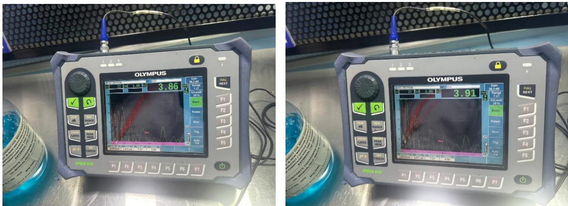
Figure 31. Ultrasonic flaw detector analysis of ABS.
