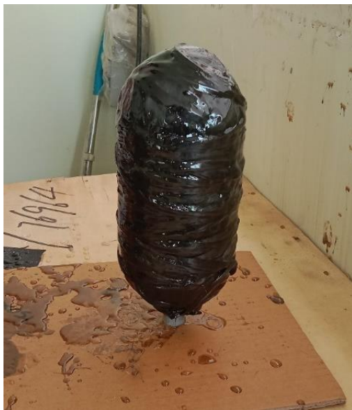
Figure 2. Wrapping of carbon fiber in ABS & PET-G cylinder.
