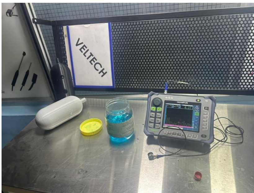
Figure 4. Ultrasonic flaw detector experimental setup
