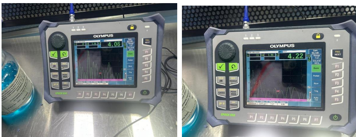
Figure 32. Ultrasonic flaw detector analysis of PET-G.
