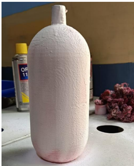
Figure 27. Dye penetrant test of PET-G.
