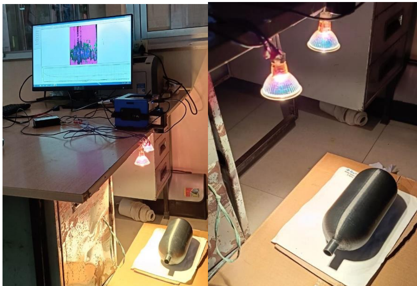
Figure 3. Multi spectra analysis experimental setup.
