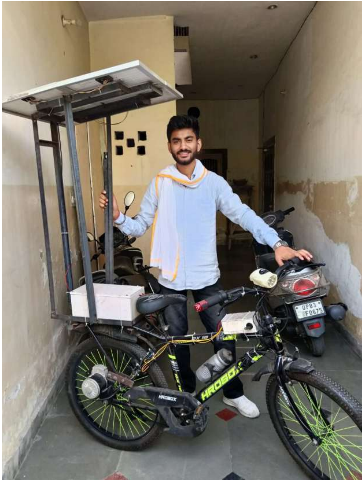
Fig. 1 Developed prototype of the solar-assisted electric bicycle.
