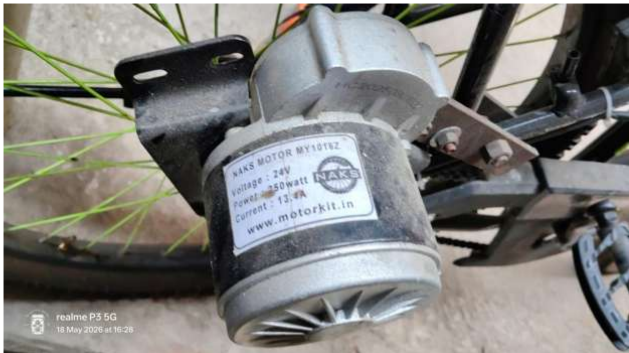
Fig. 5 24 V, 250 W brushed DC geared motor mounted on the bicycle frame.
