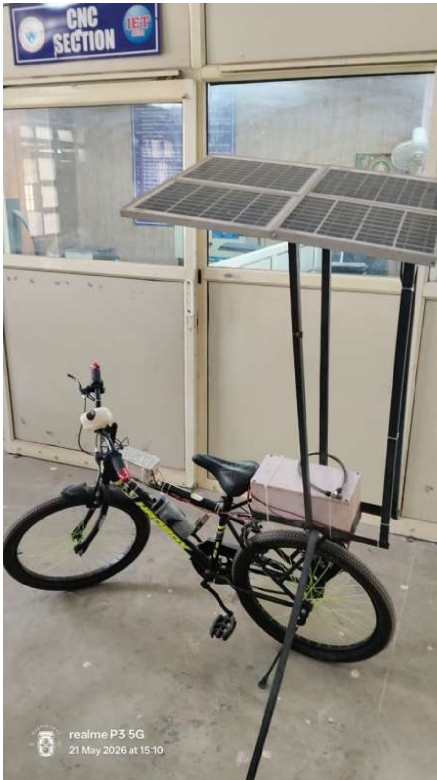
Fig.2 Fabricated solar-assisted electric bicycle during outdoor experimental testing.
