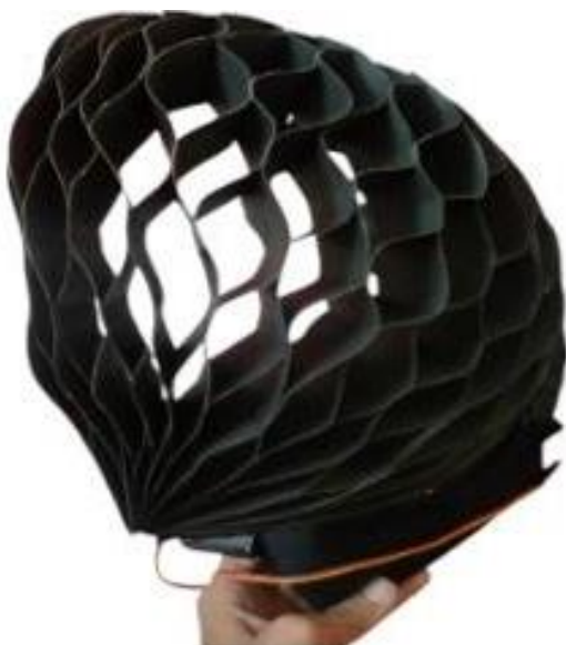
Figure 8. Honeycomb structure of helmet.
