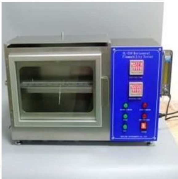
Figure 8. Horizontal Flammability Tester.
