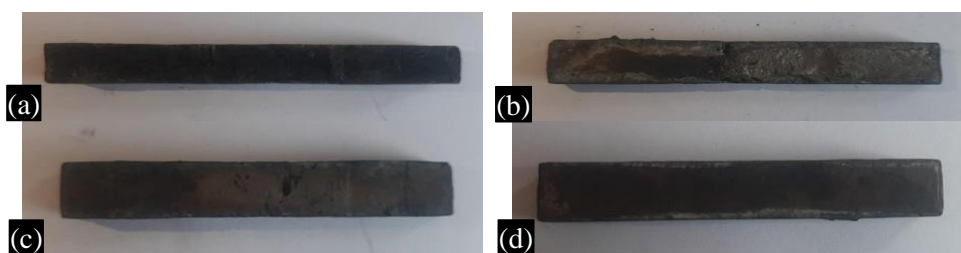
Figure 9. Horizontal flammability test specimens, (a) Carbon fiber, (b) 50% carbon fiber with 50% silicon carbide, (c) 40% carbon fiber with 60% silicon carbide, (d) 30% carbon fiber with 70% silicon carbide
