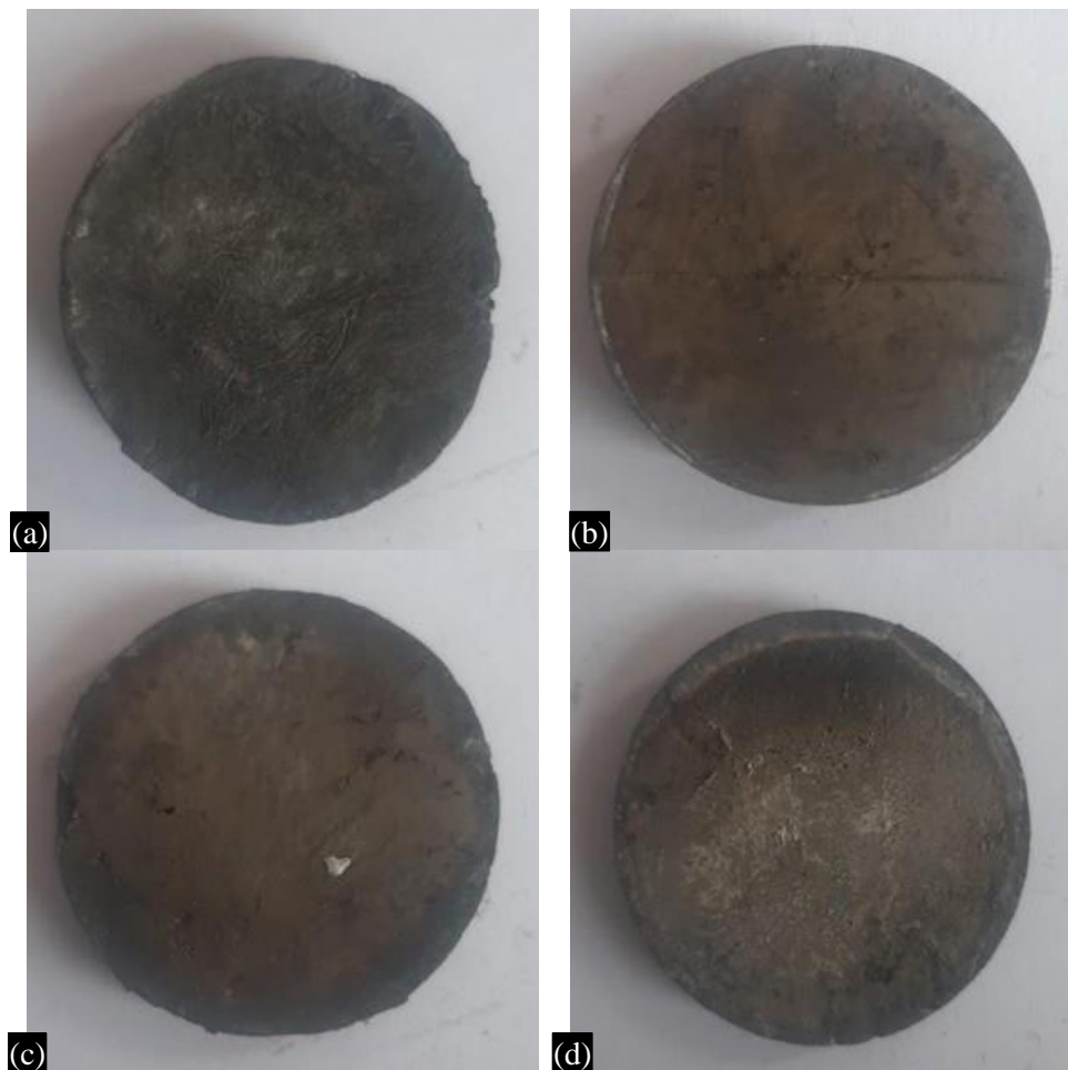
Figure 5. Thermal conductivity specimen as per ASTM E1530, (a) Carbon fiber alone, (b) 30% carbon fiber with 70% silicon carbide, (c) 40% carbon fiber with 60% silicon carbide, (d) 50% carbon fiber with 50% silicon carbide
