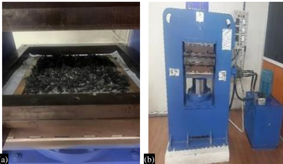
Figure 3. Compression Moulding, (a) Mould placed inside the compression moulding, (b) Mould pressed against fixed plate
