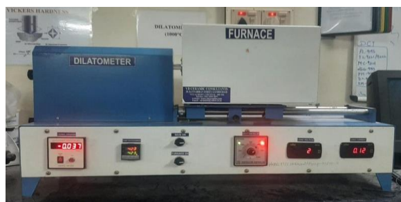
Figure 6. Dilatometer for thermal expansion.
