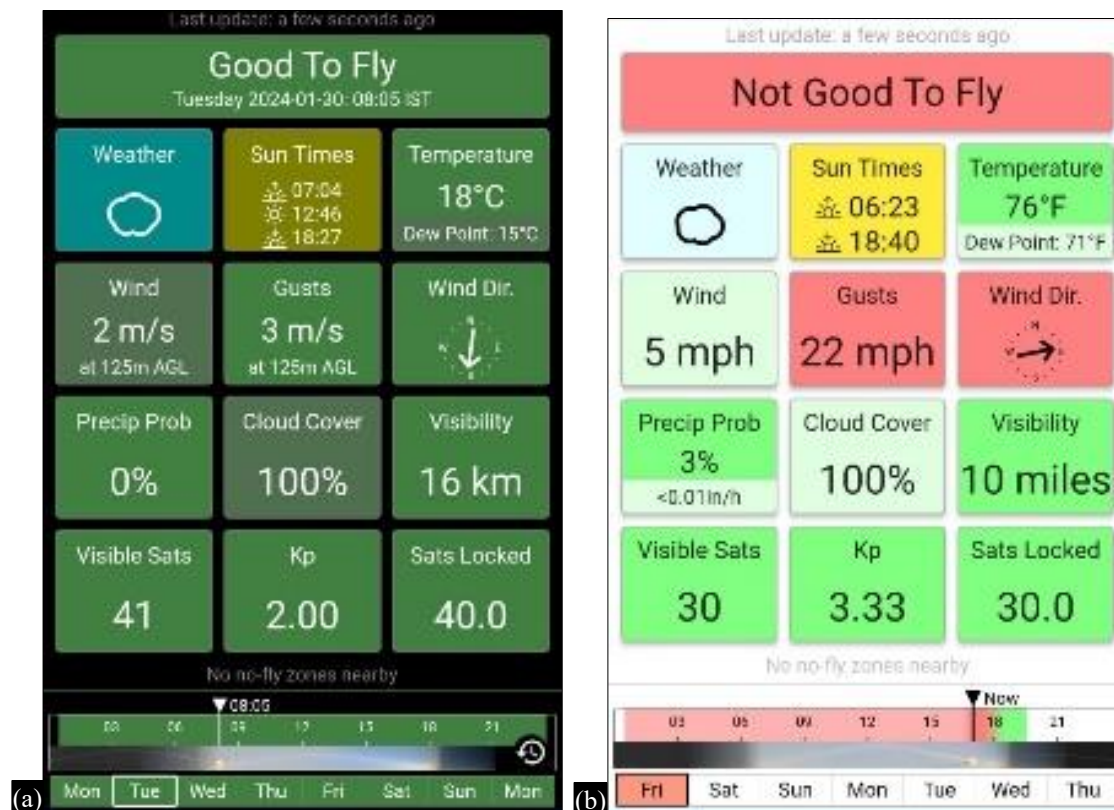
Figure 6. Conditions for pre-flight check: (a) good to fly; (b) Not good to fly.
