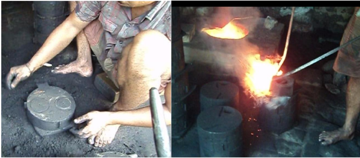
Fig.-2: Current Scenario for Non-Ferrous Foundry (a) Pattern making with bare hand, (b) Liquid Metal Pouring without precaution
