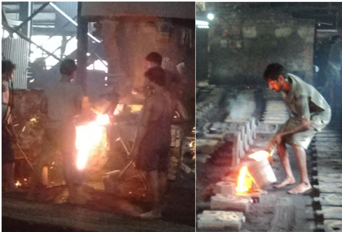
Fig.-3: Current Scenario for Ferrous Foundry(a) Melting of CI in Furnace, (b) Liquid Metal Pouring
