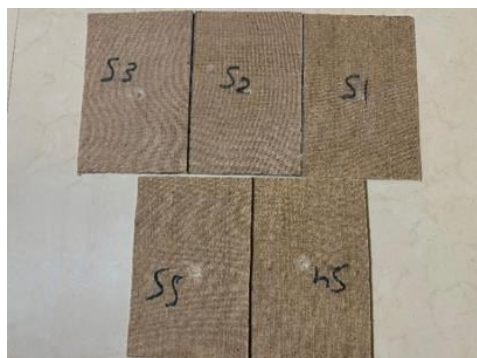
Figure 24. Hybrid linen and glass fiber composite specimens for impact test at 60°C temperature.
