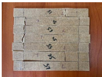
Figure 27. Linen fiber composite specimens for tensile test at 70°C temperature.
