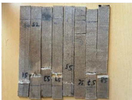
Figure 7. Hybrid linen and glass fiber composite specimens for tensile test at room temperature.
