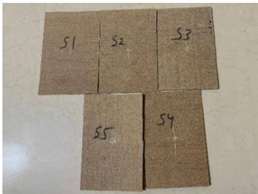
Figure 10. Linen fiber composite specimens for impact test at room temperature.
