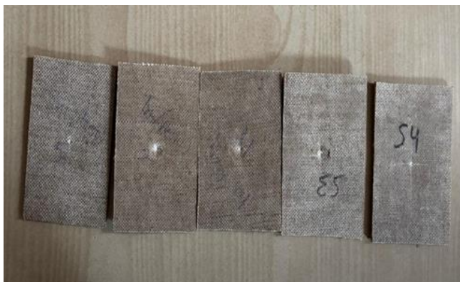
Figure 21. Hemp fiber composite specimens for impact test at 60°C temperature.
