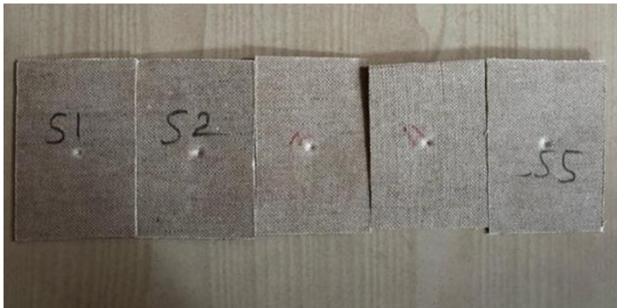
Figure 23. Hybrid hemp and glass fiber composite specimens for impact test at 60°C temperature.
