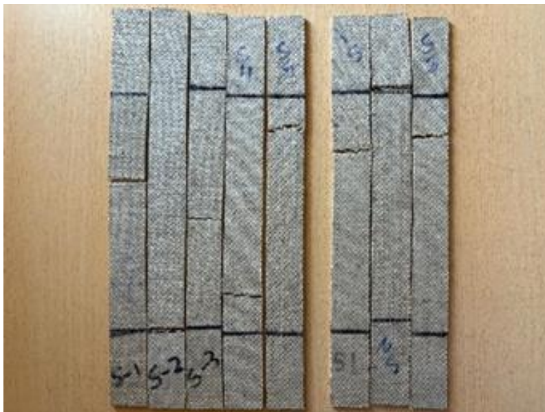
Figure 1. Hemp fiber composite specimens for tensile test at room temperature.
