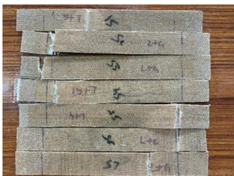
Figure 31. Hybrid linen and glass fiber composite specimens for tensile test at 70°C temperature.
