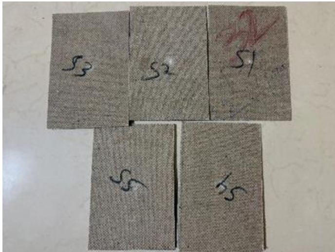
Figure 11. Hybrid hemp and glass fiber composite specimens for impact test at room temperature.
