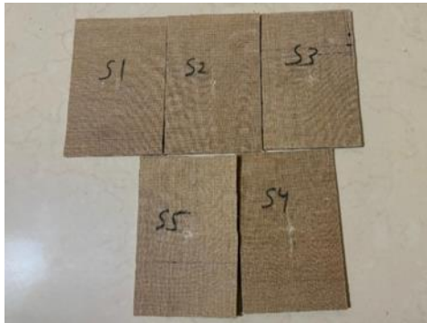
Figure 22. Linen fiber composite specimens for impact test at 60°C temperature.
