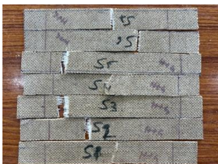
Figure 29. Hybrid hemp and glass fiber composite specimens for tensile test at 70°C temperature.
