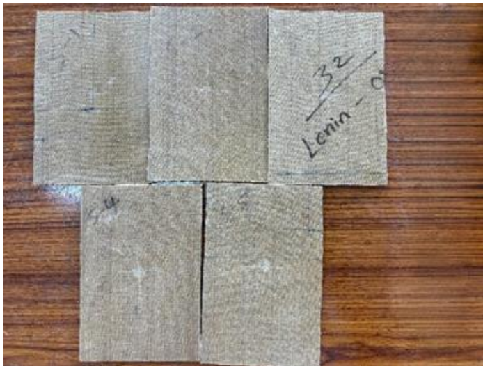
Figure 34. Linen fiber composite specimens for impact test at 70°C temperature.
