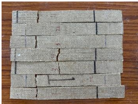
Fig 13. Hemp fiber composite specimens for tensile test at 60°C temperature.
