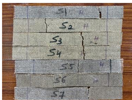
Figure 25. Hemp fiber composite specimens for tensile test at 70°C temperature.
