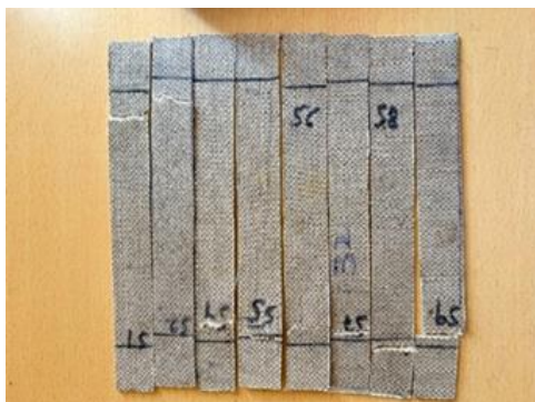
Figure 5. Hybrid hemp and glass fiber composite specimens for tensile test at room temperature.
