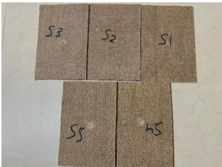
Figure 12. Hybrid linen and glass fiber composite specimens for impact test at room temperature.
