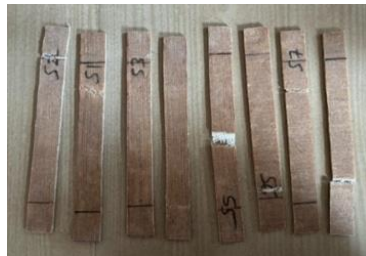
Figure 19. Hybrid linen and glass fiber composite specimens for tensile test at 60^\circ\text{C} temperature.
