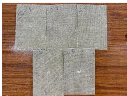
Figure 35. Hybrid hemp and glass fiber composite specimens for impact test at 70^\circ\text{C} temperature.
