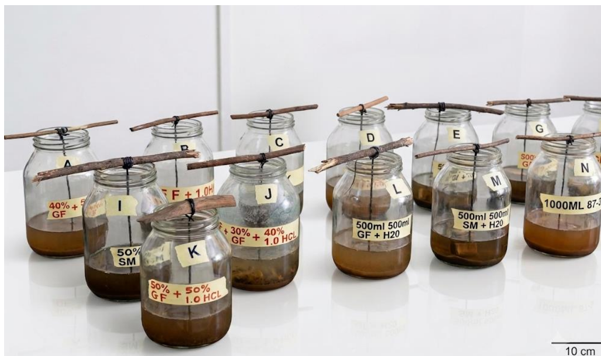
Figure 1. Weight losses and corrosion rate experimental setup at room temperature.
