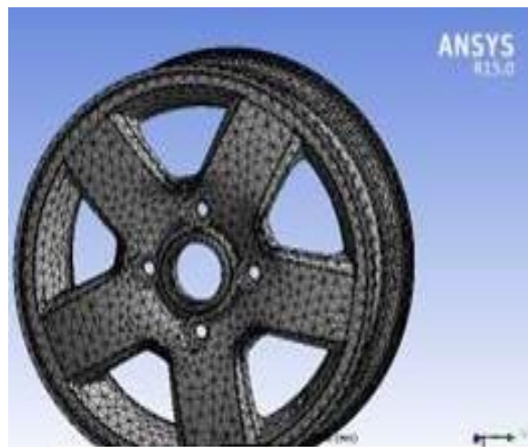
Figure 4. Alloy wheel: mesh model.
