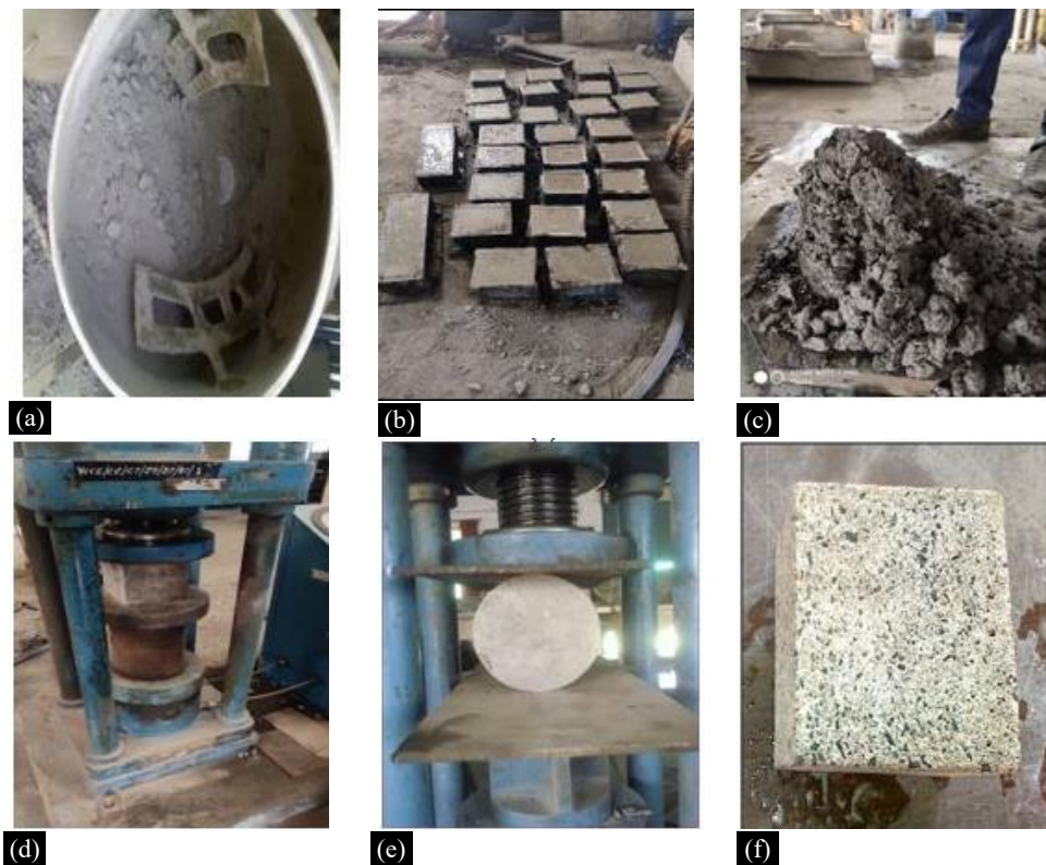
Figure 1. [a] Mixing, [b] Casting, [c] Workability, [d, e, f] concrete's mechanical properties.
