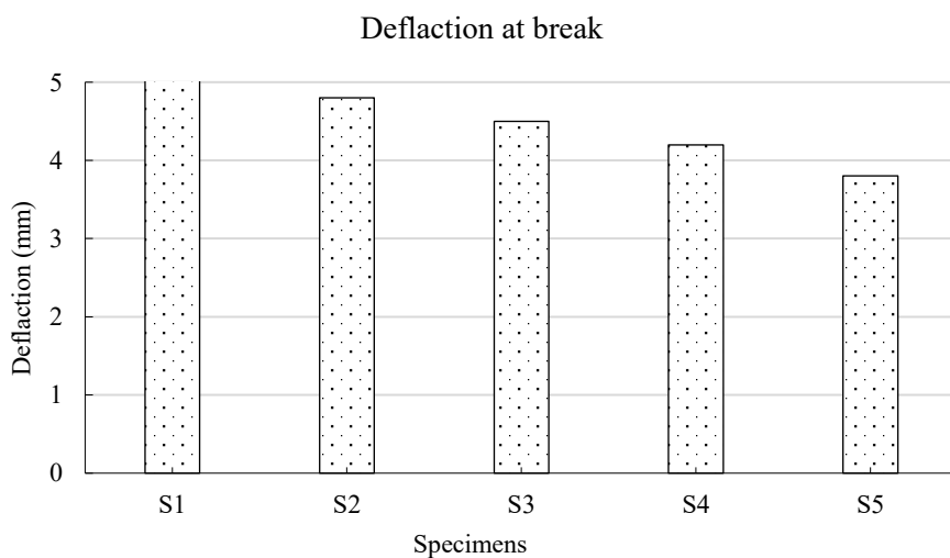
Figure 7. Deflection at Break in mm for Different Composite Specimens.
