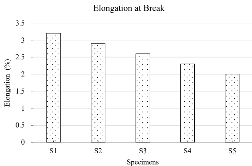
Figure 4. Elongation (%) at Break for Different Composite Specimens.
