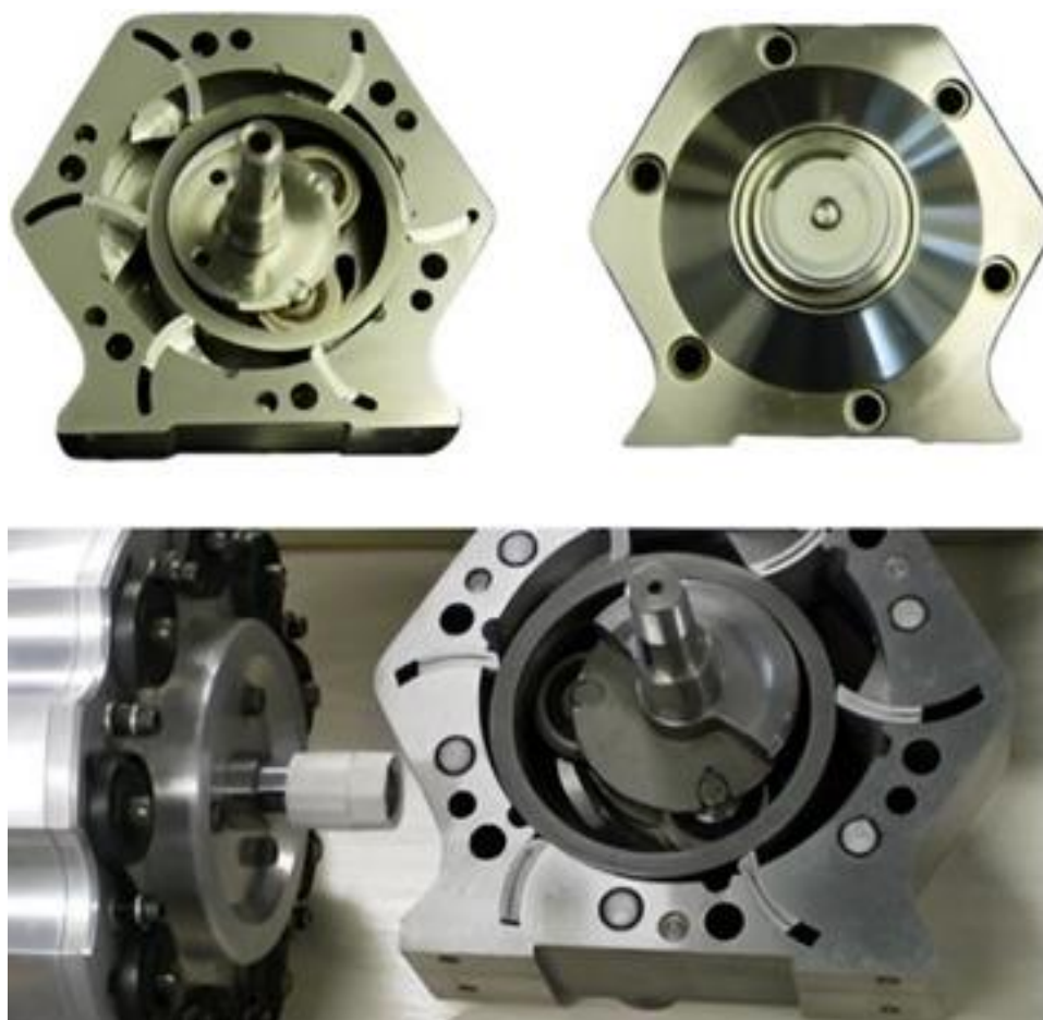
Figure 5. Di Pietro motor 6-cylinder expansion motor [23].
