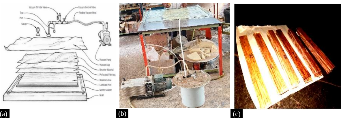
Figure 1. (a) Line diagram, (b) Experimental setup for vacuum bagging process, (c) alkali-treated specimens and untreated alkali specimens.
