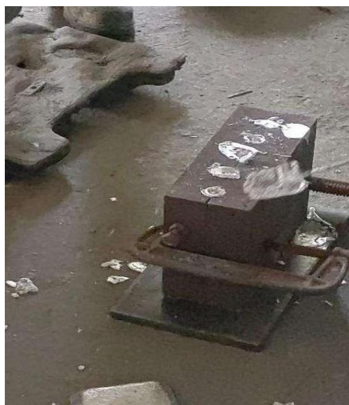
Figure 4. Molten material poured into the mould.
