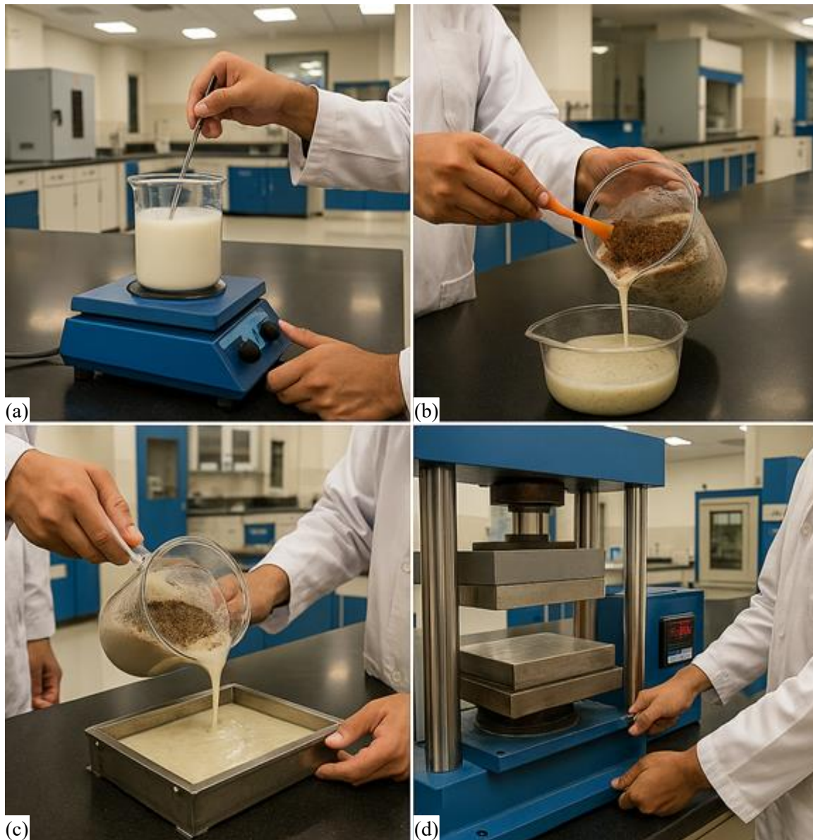
Figure 1. Stepwise fabrication process of crosslinked bio-polymer composites reinforced with marine algal microfibers and agro-waste fillers: (a) preparation of starch–PVA polymer solution with citric acid and glycerol, (b) dispersion of marine algal microfibers and agro-waste fillers into the polymer solution, (c) casting of the composite slurry into stainless steel molds, and (d) hot press curing of the composite sheets to induce crosslinking and consolidation.
