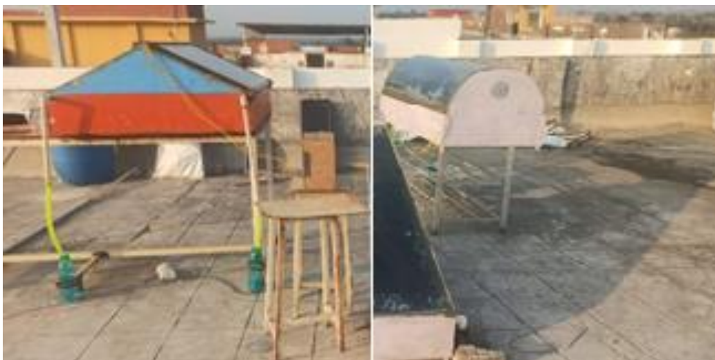
Figure 1. Experimental setup of SCSS (semi-cylindrical solar still with iron wick) and DSSS (double-slope solar still with jute wick).
