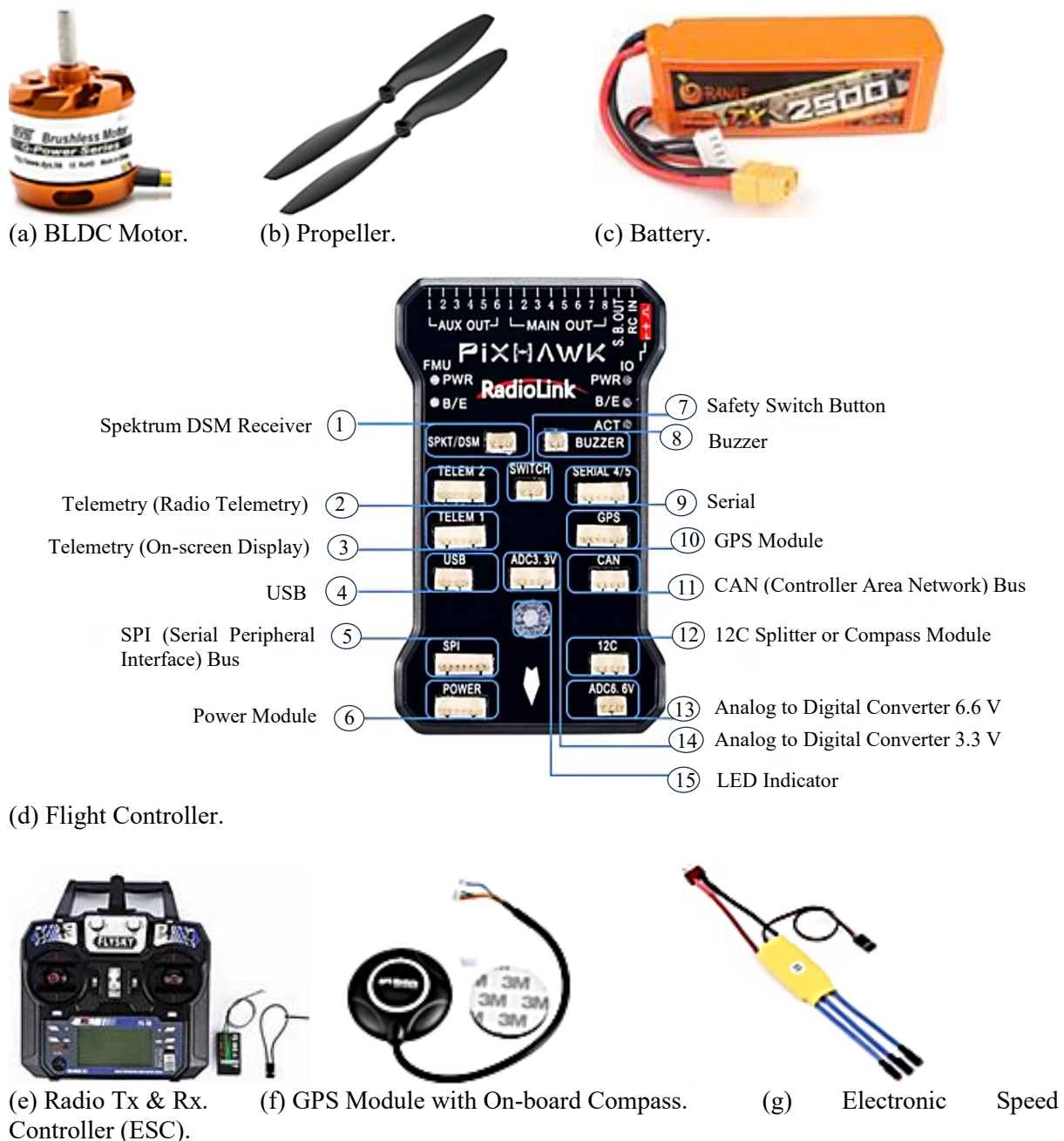
Figure 1. Components of Drone for Constructions.
