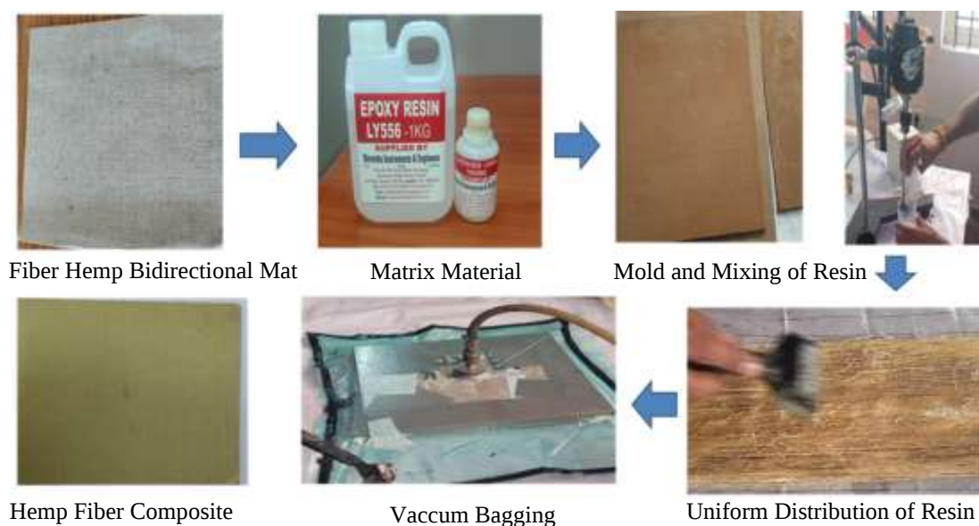
Figure 2. Hand Lay-up and vacuum-bagging fabrication process.
