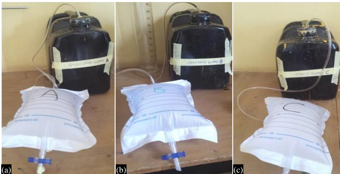
Figure 3. Digesters feeding the urine bags with biogas.
