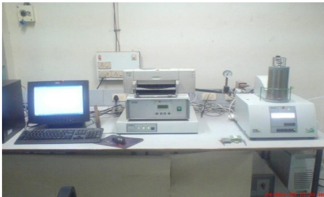
Figure 1. Simultaneous thermal analyzer by NETZSCH, Model STA 449 C.
