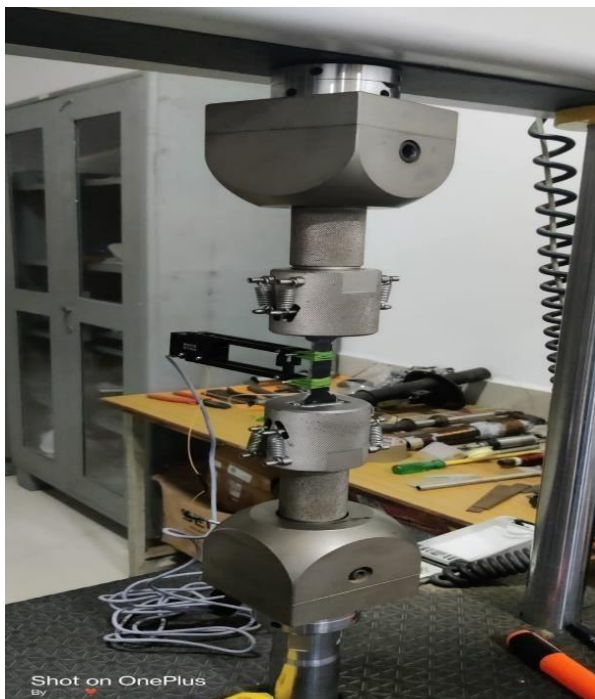
Figure 7. Tensile test specimen in UTM machine.
