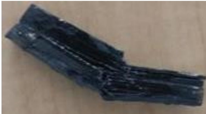
Figure 11. Specimen after Charpy test Bending Examination.
