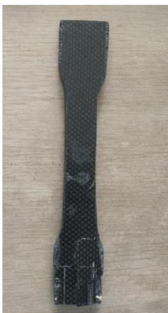
Figure 9. Specimen after Tensile test.
