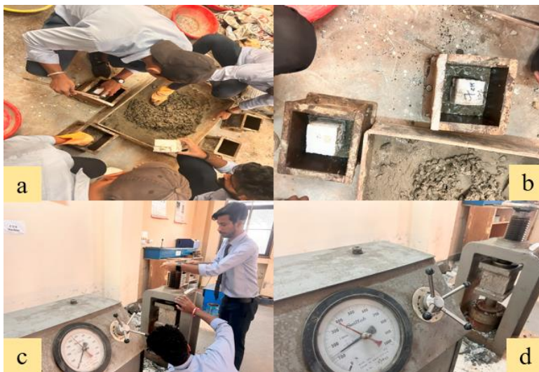
Figure 1. (a) Preparation of concrete, (b) casting of M20 concrete with different sizes of plastic cubes, (c) setup of concrete cube specimen in compression testing machine (CTM), and (d) failure load for each specimen is noted.
