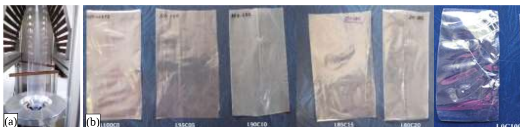
Figure 3. (a) Blown Film Preparation (b) Blown film samples of L 100 C 0 , L 95 C 05 , L 90 C 10 , L 85 C 15 , L 80 C 20 and L 0 C 100 .
