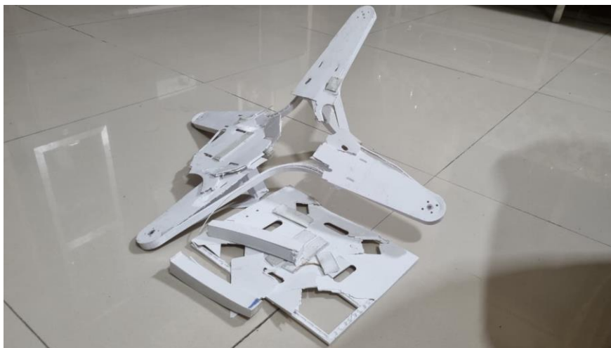
Figure 3. Structure frame 1 (White Frame) structural failure after hard landing on flight 10. The use of solid infill landing gears (100% infill) did not provide any benefit in terms of weight increase and reduction in critical load paths.
