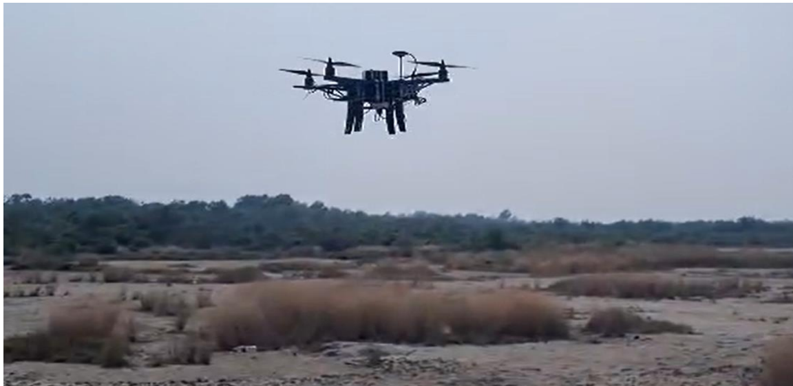
Figure 5. Frame 2 when it is at flight. Flown successfully 40+ times with no structural failures and showed variable infill, layer orientation and acetone bonding strategies to be effective.
