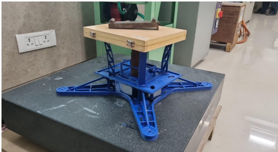
Figure 2. Masses that are added to the acetone evaporation in order to counter thermal warping forces and to ensure that the surface is flat during interdiffusion of the polymer chains. Curing time: 4–6 hours minimum.
