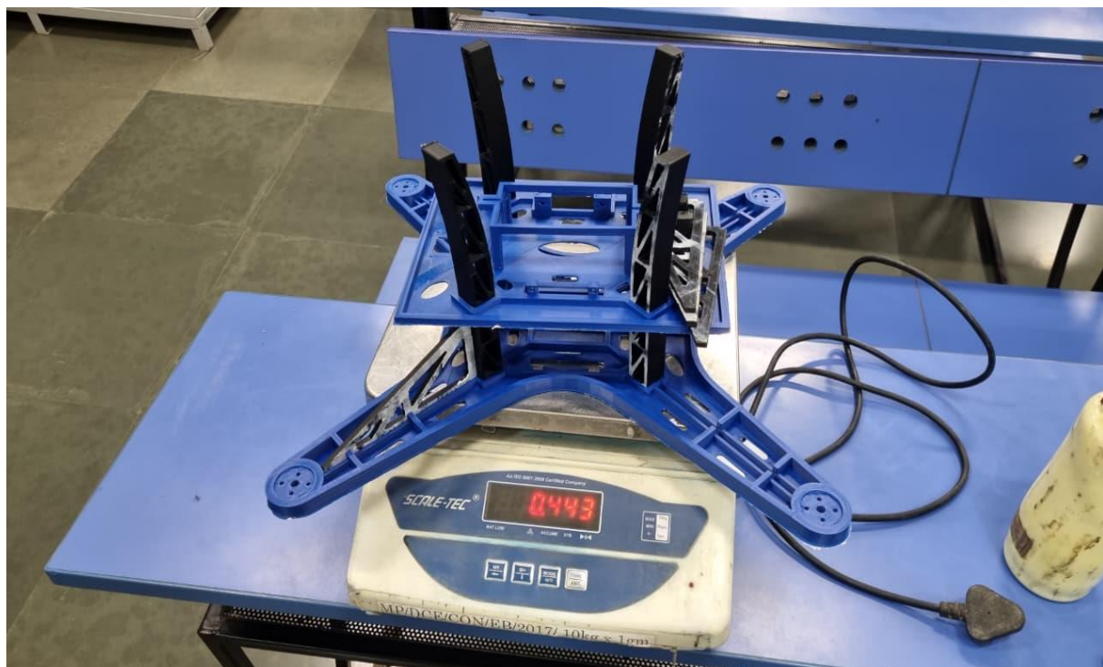
Figure 4. Total assembly weight Frame 2 (Blue Frame): 443 grams. Variable infill strategy (60% arms/landing gears, 20% body) had 7g reduction in weight over Frame 1 whilst still being structurally intact after 40+ flights.
