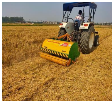
Figure 3. Rotary mulcher during operation.
