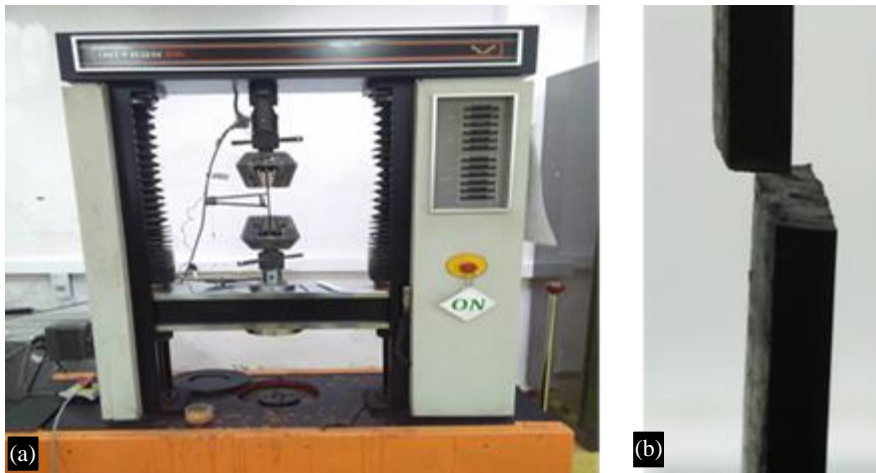
Figure 4. (a) Test setup (b) view of a fractured specimen.
