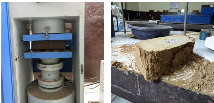
Figure 1. Compression test for 0.1% Recron fiber reinforced block.
