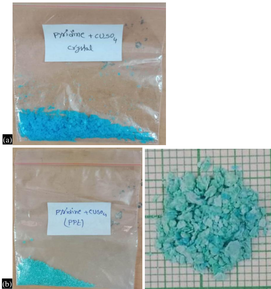
Figure 1. Photographs of (a) blue pyridine copper sulfate crystal; (b) green pyridine copper sulfate precipitate.
