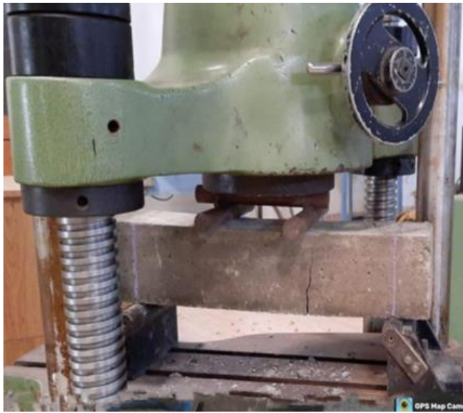
Figure 3. Test Arrangement for loading and cracking.
