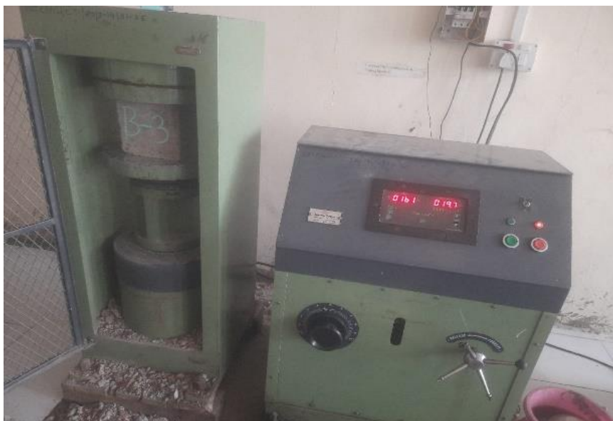
Figure 2. Test arrangement for crushing strength test.
