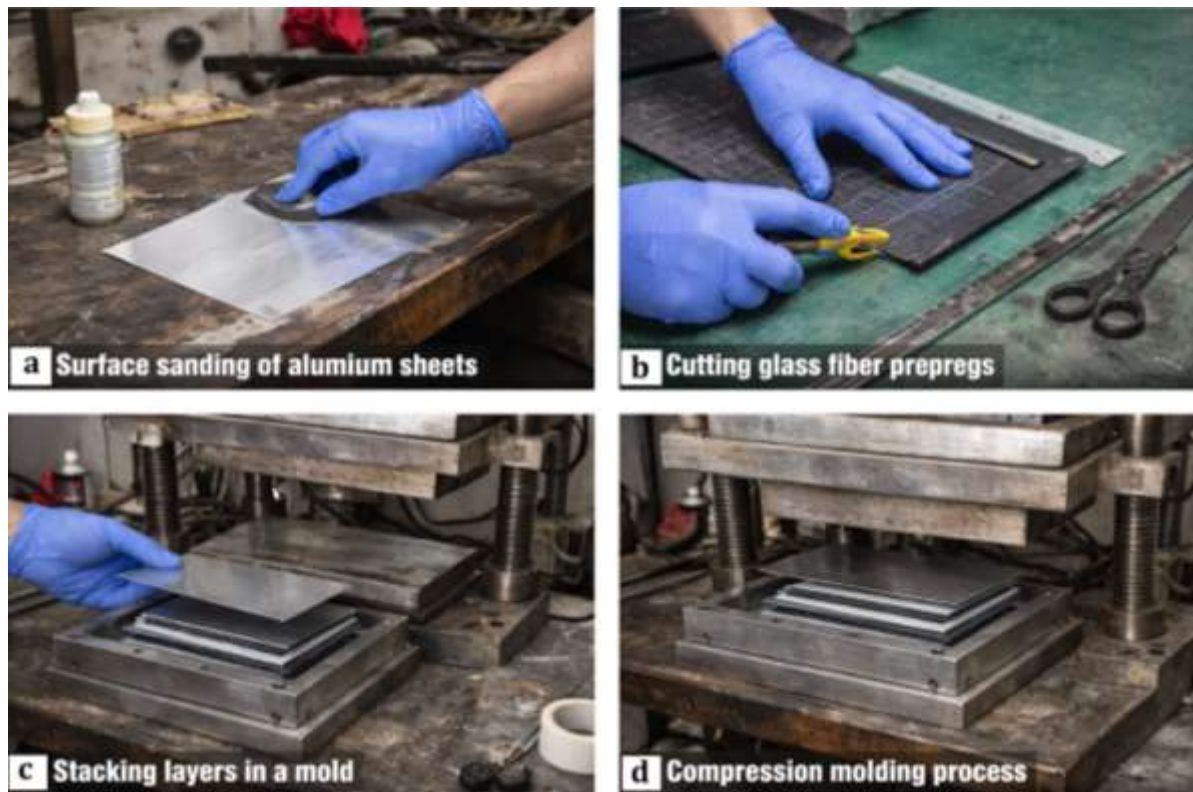
Figure 1. Preparation of metal–polymer hybrid laminate; (a) Surface preparation of aluminum sheets (b) Cutting of glass fiber prepregs (c) Stacking of laminate layers (d) Hot compression molding of the hybrid laminate
