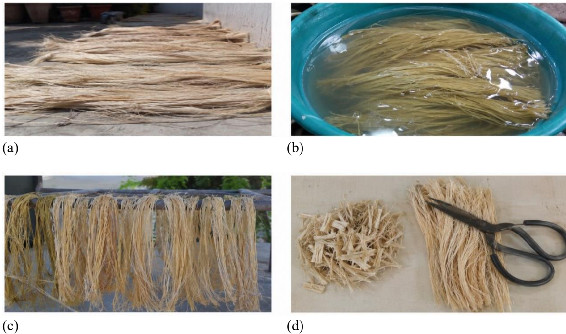
Figure 4. Manufacturing stages of unidirectional areca/PALF hybrid composite.
