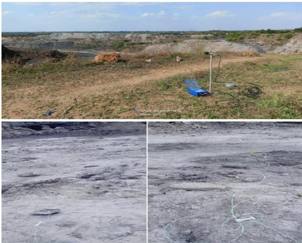
Figure 5. Ground vibration monitoring setup.
