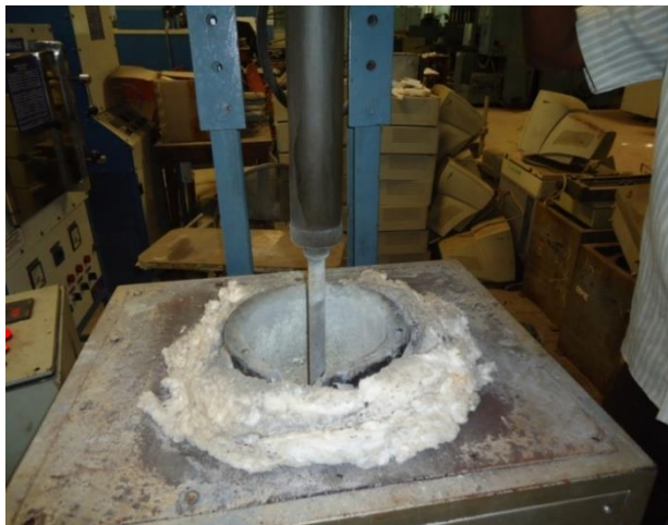
Figure 3. Electrical Resistance Furnaces with a Stirring Assembly.
