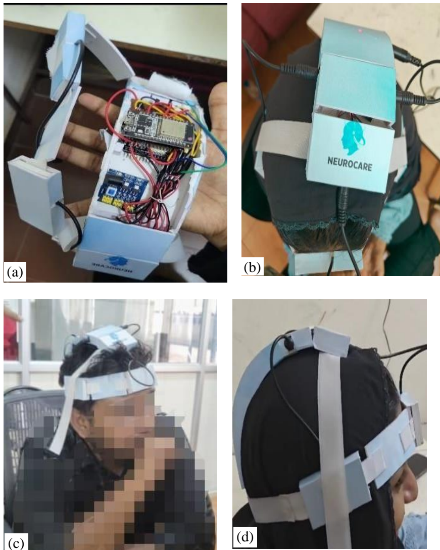
Figure 4. (a) Internal view of the NeuroCare smart helmet, showcasing the internal components, including the microcontroller, and wiring for the vibration motors. (b) Top view of a user wearing the NeuroCare smart helmet. (c) Front view of a user testing the NeuroCare smart helmet. (d) Side View of a user wearing the NeuroCare smart helmet during a therapy session.
