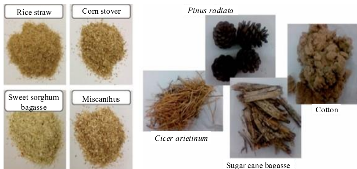
Figure 1. Suitable biomass for the industrial scale production of levulinic acid [Adapted with permission from 26, 27].
