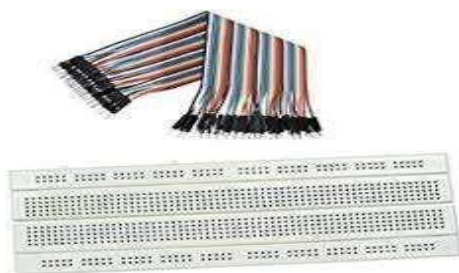
Figure 7. Connecting wires and breadboard.
