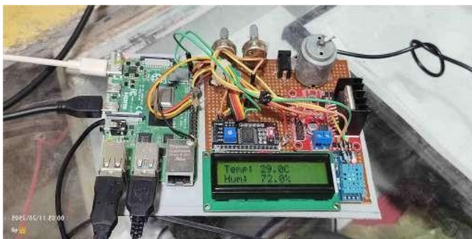
Figure 10. Real-time temperature and humidity monitoring on LCD.
