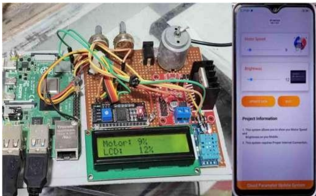
Figure 9. Motor speed and LCD brightness displayed on LCD and android app.
