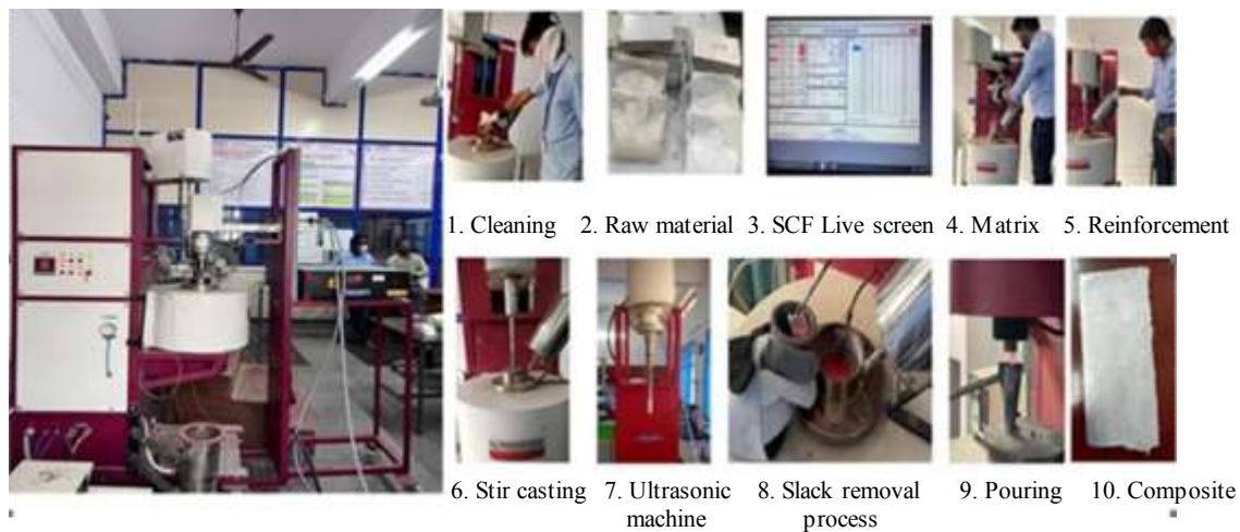
Figure 1. Schematic representation of ultrasonic vibration-assisted stir casting process
