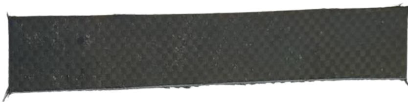
Fig. 4.2.1. Flexural Test Specimen.
