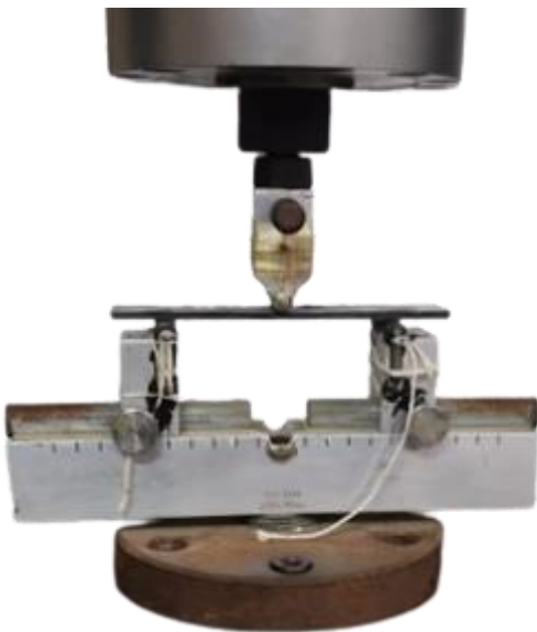
Fig. 3.2.1. Three Point Flexural Test Rig.
