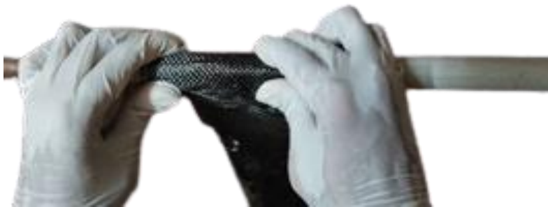
Fig. 2.5.1. Fabricating of Drive Shaft.
