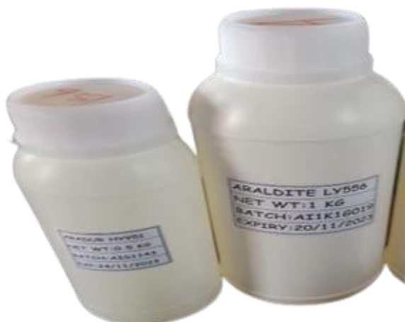
Figure 2.3.1: Resins and Hardener for Reinforcement Carbon Fiber.
