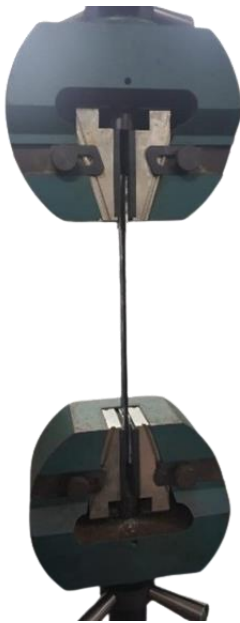
Fig. 3.1.1. Tensile Testing Rig for Composites.
