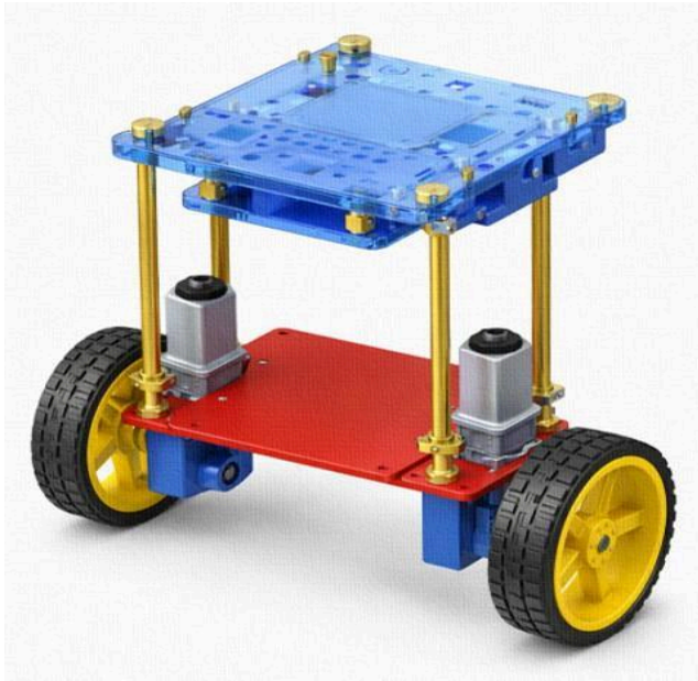
Figure 1. Inverted pendulum model of the two-wheeled self-balancing robot.
