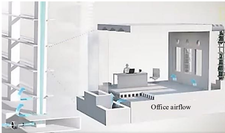
Figure 10. Air circulation inside the office through the chimney Source: Termite inspiration for a self-cooling building , www.btp-cours.com [14].
