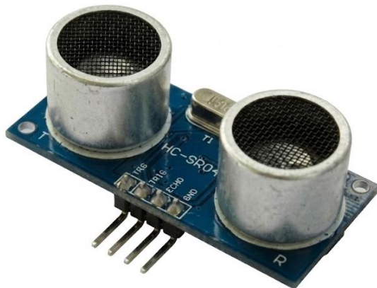
Figure 3. Ultrasonic sensor (HC-SR04).
