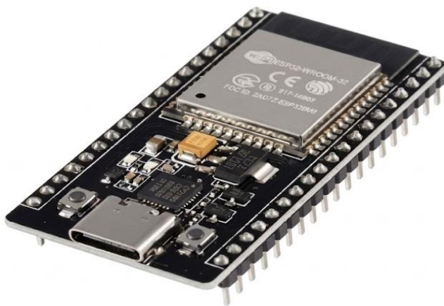
Figure 2. ESP32 microcontroller board.
