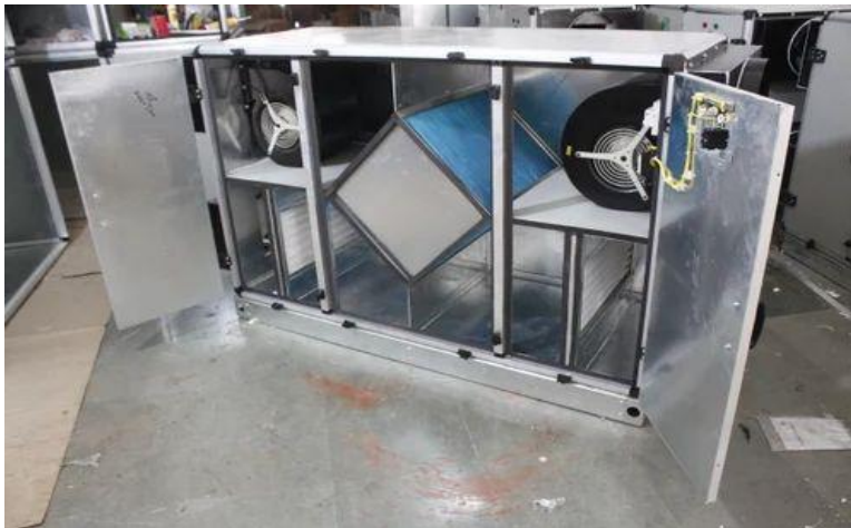
Figure 4. Plate heat exchanger used in Air handling unit.
