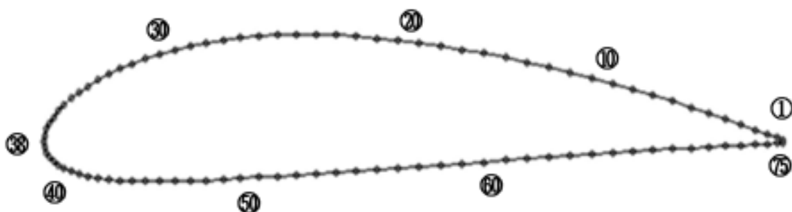
Figure 1. The node points of airfoil.
