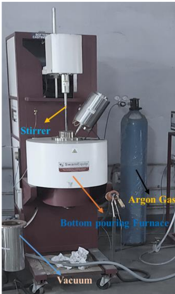
Figure 2. Experimental setup – Vacuum Assisted Stir Casting.
