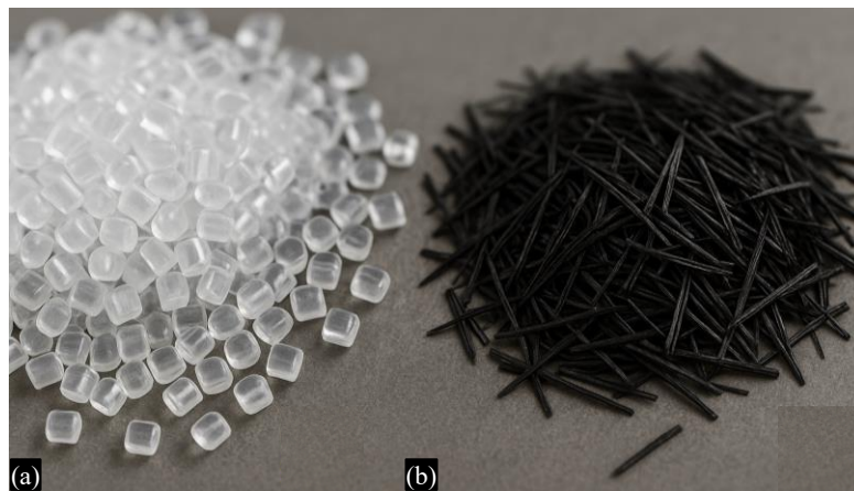
Figure 1. Visual representation of (a) PETG pellets and (b) Short chopped carbon fibers.
