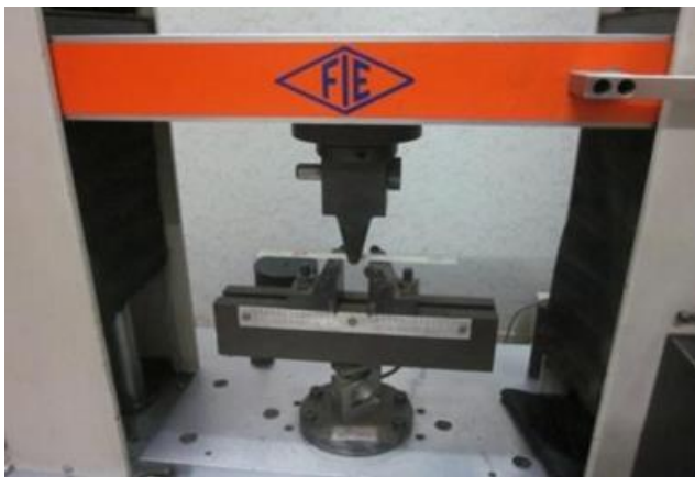
Figure 8. (UTM flexural strength test machine with ASTM-D790 standards) [20].
