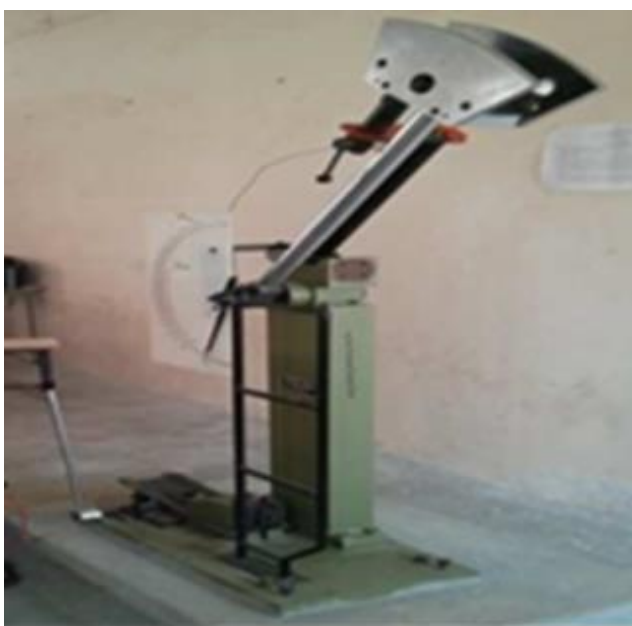
Figure 9. (Impact test machine with ASTM-A370 standards) [21].
