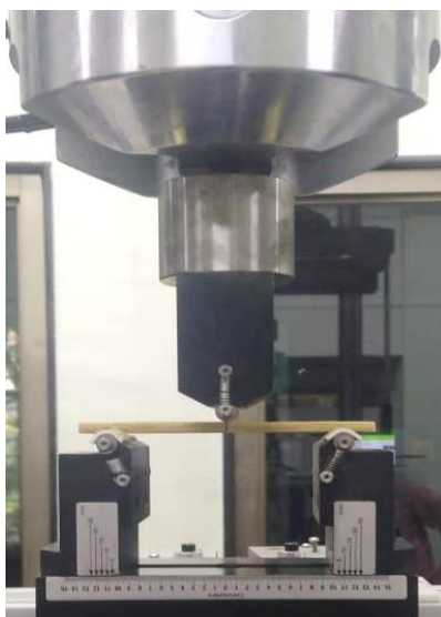
Figure 4. Flexural test setup UTM.
