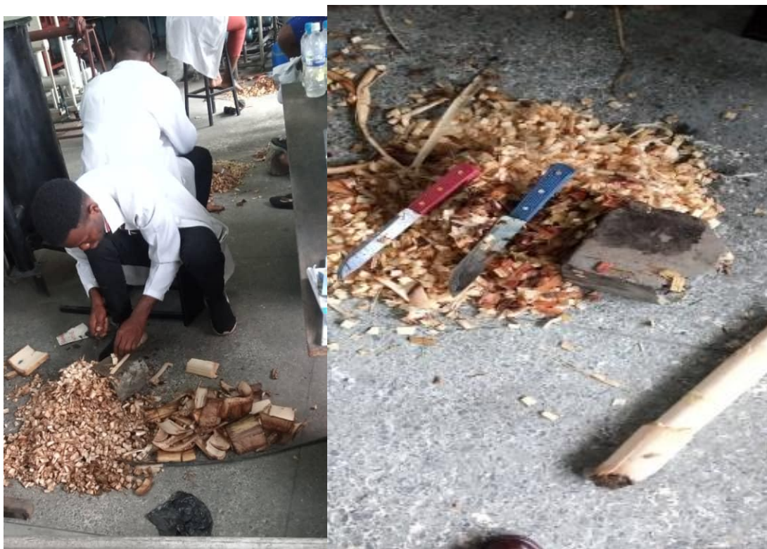
Figure 15. Manuel Approach of Plantain and Banana Stem Size Reduction.
